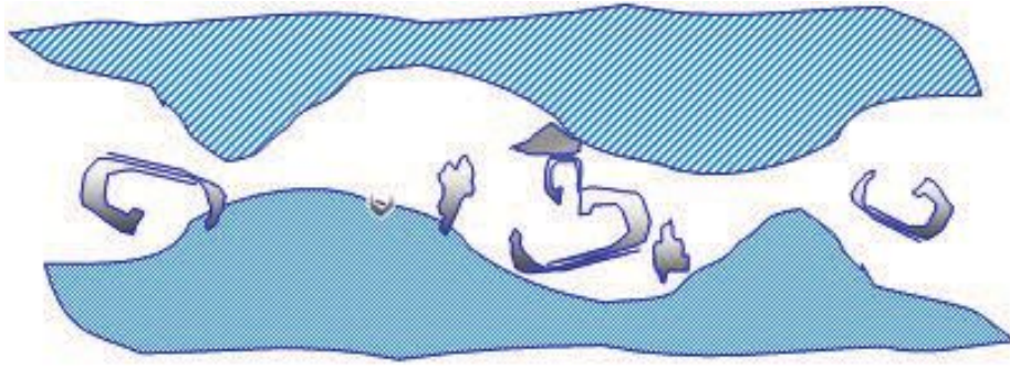
Figure 1 | These third-body wear particles swim around in our lubricants and can arise from initial manufacture of the lubricant.
